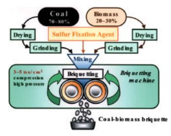
Fig. 2 Production flowchart of the coal-biomass briguette.
