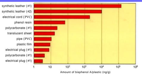
Fig. 3 Levels of bisphenol A leached from various plastic wastes.
