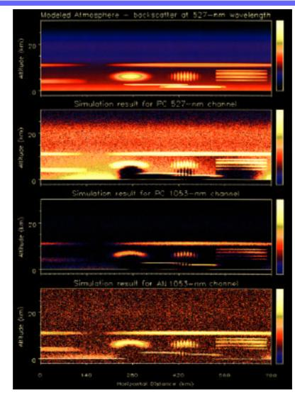
Fig. 2 Example of a simulation study. Modeled backscatter by clouds and aerosols (top panel), and simulated signals from the 3 detection channels (lower 3 panels).
