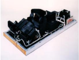
Improved Limb Atmospheric Spectrometer (ILAS) flight model (without cover).
