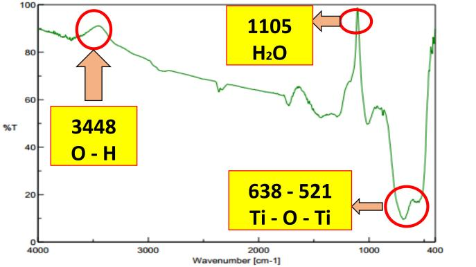
Figure 6. The Fourier transform infrared spectra of TiO<sub>2</sub> material
