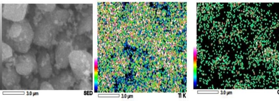
Figure 5. The mapping images of a) TiO<sub>2</sub> material consisting of b) oxygen and c) titanium elemental particles
