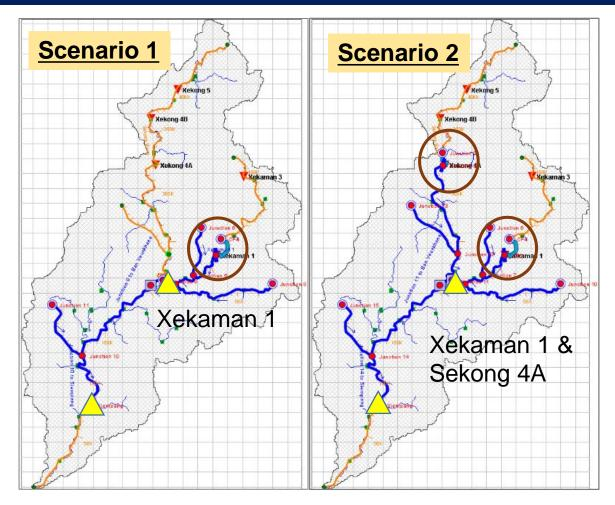
Reservoir operation schematic for the Xekaman 1 hydropower dam "Scenario 1" (left) and Xekaman 1 and Sekong 4A hydropower dams "Scenario 2" (right)
