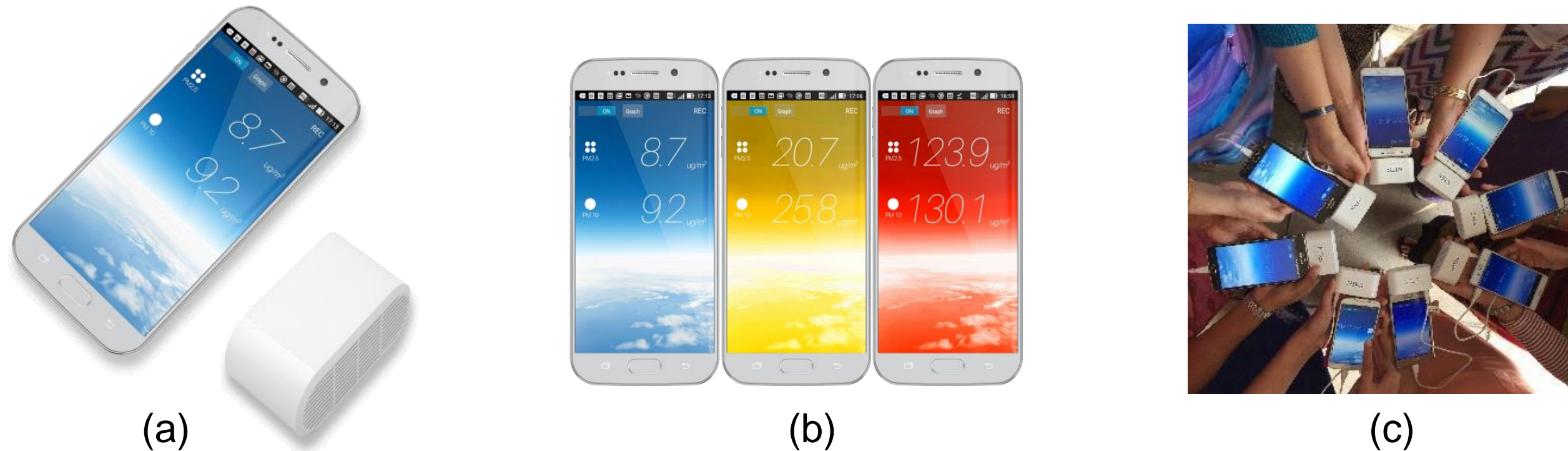
Fig 2 (a). Pocket PM 2.5 Sensor, a smart phone with android system, (b) color variations for level of PM 2.5 concentration and (c) recording PM 2.5 at the starting point for 8 tracks.
