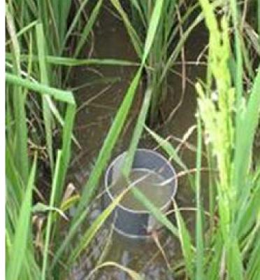
Field water tube made up of PVC. Note the holes on all sides
