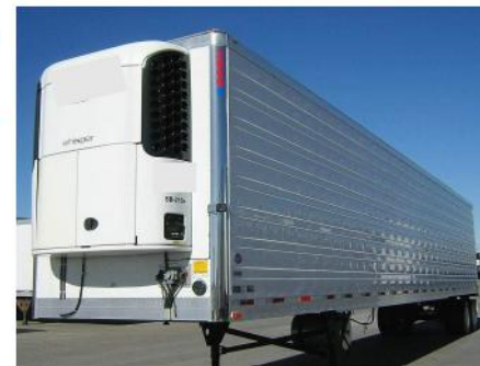
Refrigerated trailer with dedicated diesel engine and cooling system
