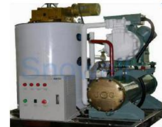
Flake ice making system for a fishing trawler
